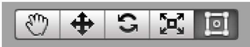
Figure 4: Mode buttons for manipulating GameObjects in the Scene View (from left to right): Pan, Translate, Rotate, Scale, Sprite.
